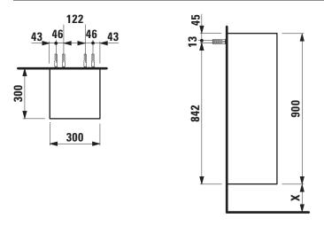
X = The exact hight must be set during installation.
